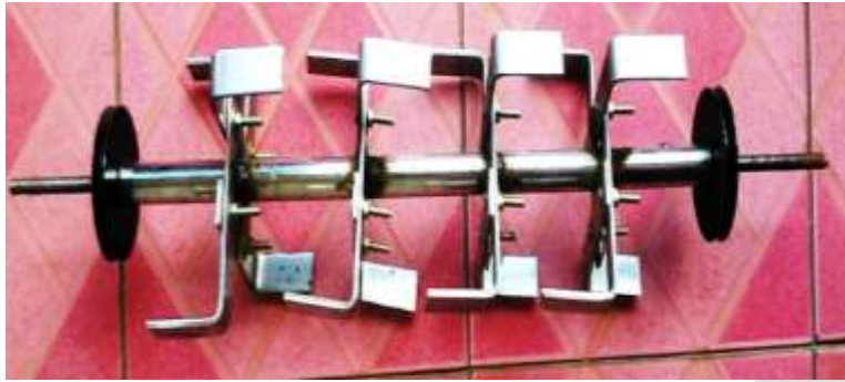
Fig-3. Tiller attachments with pulley system
