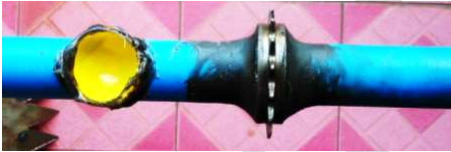
Fig-8. Spherical cavity for seed carrying
