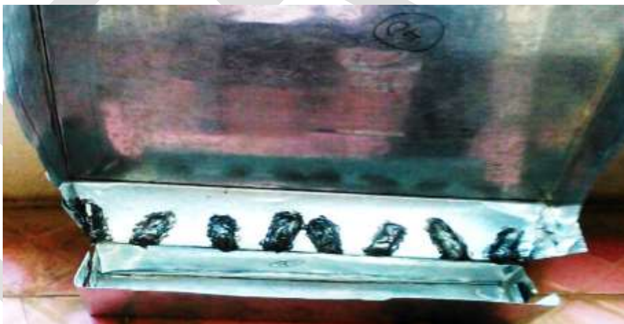
Fig-7. Funnel attachment with lanes of seed flow
