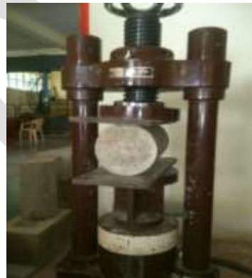
Fig 4: Split Tensile Strength Test
