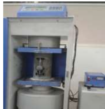
Fig 6: Modulus of Elasticity (E) Test
