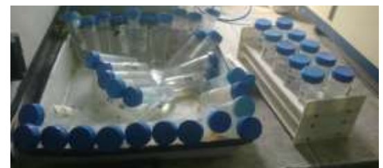
Fig. 1: Culture tubes with PTTE-lined screw caps
