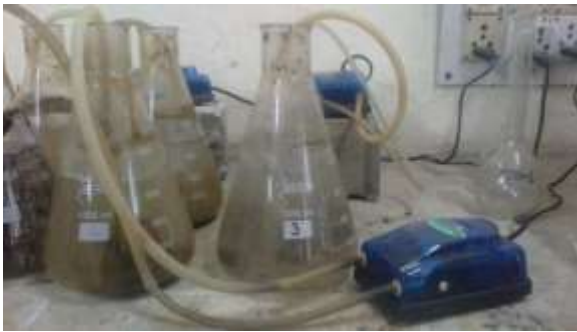
Fig. 4: Reactor when kept on aeration
