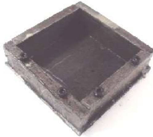
Figure 4.3 Bending Sample mould
