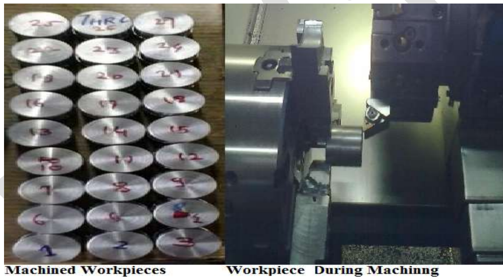
Fig.1 Machined Workpieces and Workpiece with cutting tool during machining
