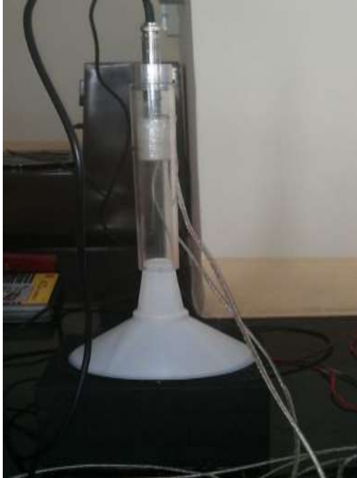
Figure 3: Resonator at the top of the acoustic generator
