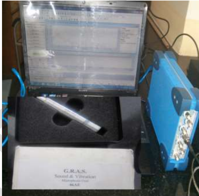
Figure 4: FFT Analyzer for pressure measurement
