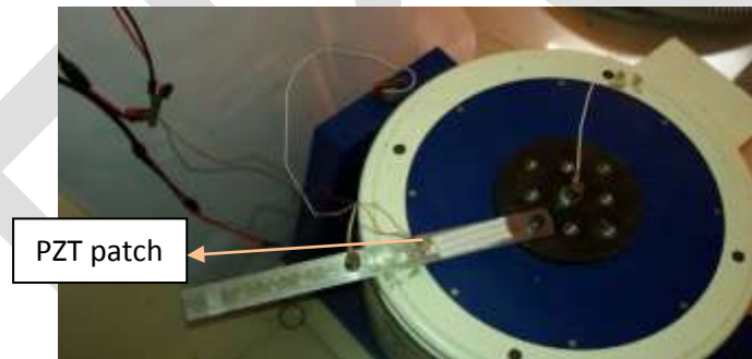
Fig. 3 mounting of beam on shaker
