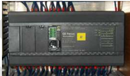
Fig. 2. Appearance GE Fanuc PLC VersaMax Micro IC200UDR164 used in the model
