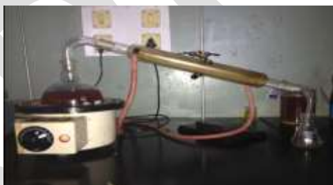
Fig 4.3: Methanol recovery through distillation
