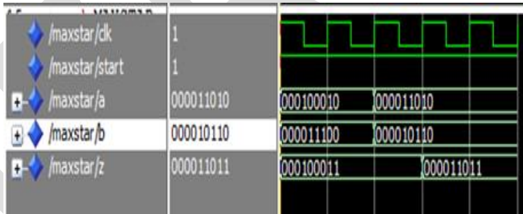
Fig 5: Output waveform of LUT Max* operation
