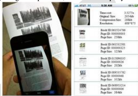
Figure1: Left: Document image capture by mobile device. Right: Document retrieve from digital library [2]
