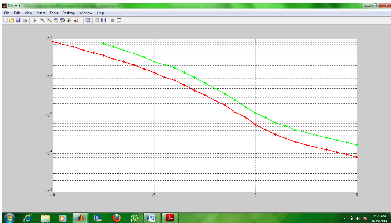
Fig: 9 BER Vs Es/No using HV1 and DM5 packets with and without Wi-Fi interfere
