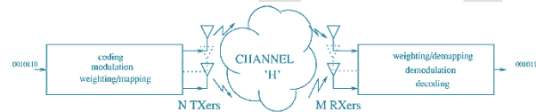
Figure 7: Diagram of a MIMO wireless transmission system. The transmitter and receiver are equipped with multiple antenna elements. Coding (STBC), modulation, and mapping of the signals onto the antennas may be realized jointly or separately.
