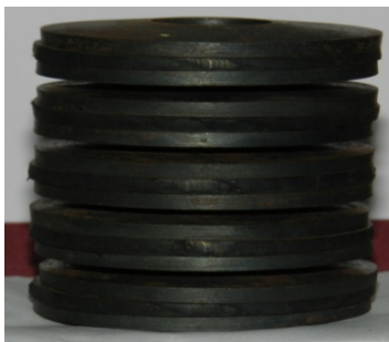
Fig. 5. Series combination of 'EPDM-EN 45' disc spring.
