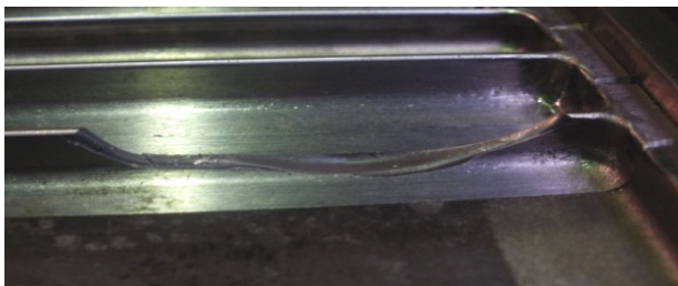
Fig. 2b. Failure of die segment.
