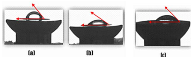
Figure 7: The pictures of sensile drops for surfaces (a) unmodified (b) plasma modified, (c) activated surfaces.
