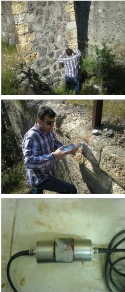
Fig. 4. In situ Schmidt test and ultrasonic wave velocity test on stone samples.
