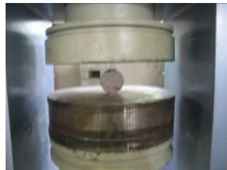
Fig. 3. Drilling out core samples, uni-axial compression and Brazilian test.
