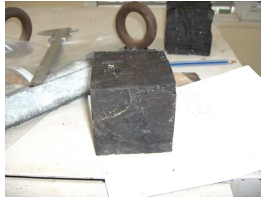
Figure 7. UCS experiments of coal sample (7×7×7 cm)
