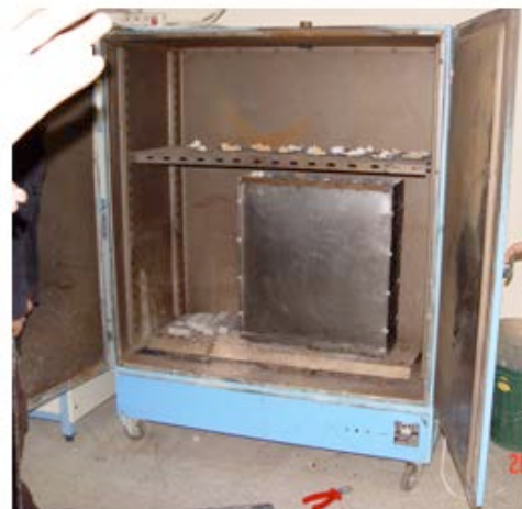
Figure 10. Mould is pressed and dried in the oven
