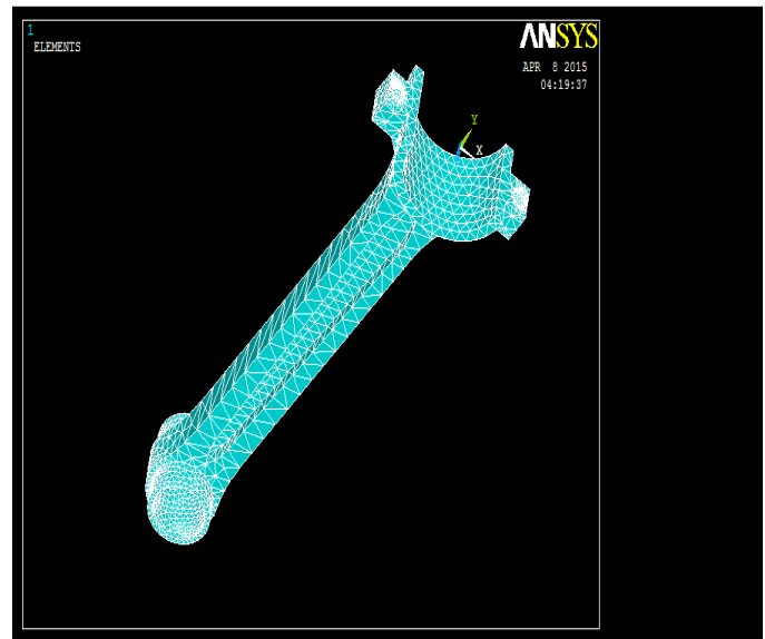
Figure 7: Meshed model of connecting rod on ANSYS
