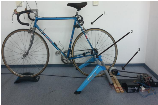
Figure 2. Bike-powered electricity generator; scavenging system – mechanical block and electric block
