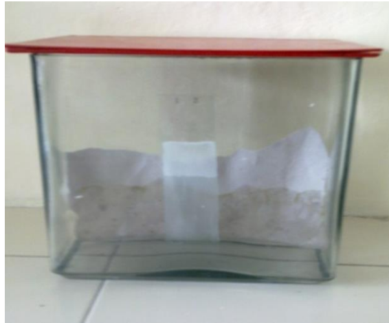
Fig 4: TLC Plate Showing Development of Chromatogram
