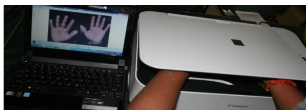
Fig 1: Canon PIXMA MP250 Inkjet photo All-in-one Printer with lap top connected to it to record the finger prints.
