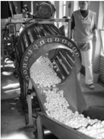
a) Cleaner to remove the coarse silk yarn spun b) Cocoons way out of the "shaken" cooker
