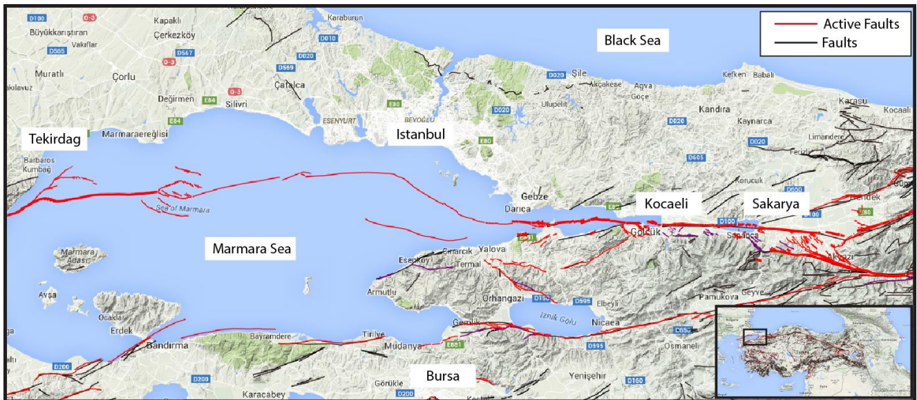
Fig. 1. Active faults segments at Marmara region with long-term seismic gaps (Emre et al., 2013).
