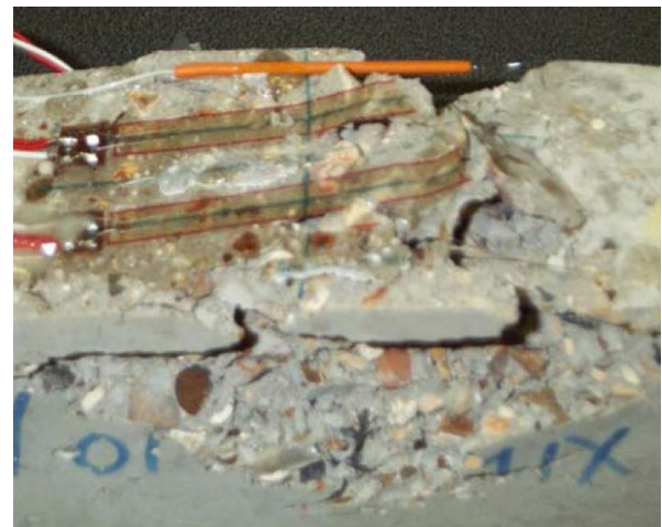
Fig. 3. Strain gauges and optical fibre sensors on failed concrete specimens.
