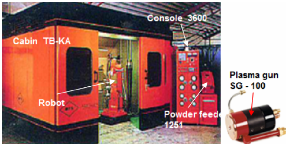
Figure 7 – APS equipment for plasma powder deposition at atmospheric pressure (Mrdak, 2010, pp.5-16)
