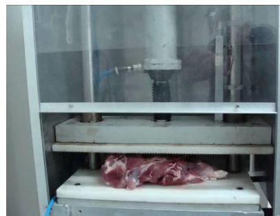
Fig. 2 - Cyclic impulsive pressing machine (food grade Teflon pads with pyramidal prongs)
