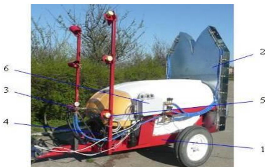
Fig. 2 – The machine for high accuracy application of phytosanitary treatments in orchards MSL [8] 1 - the frame with rolling system; 2 - the spraying device; 3 - the liquid installation; 4 - the angular gear; 5 - the detection system of the presence / absence of the tree canopy; 6 - the automatic control system
