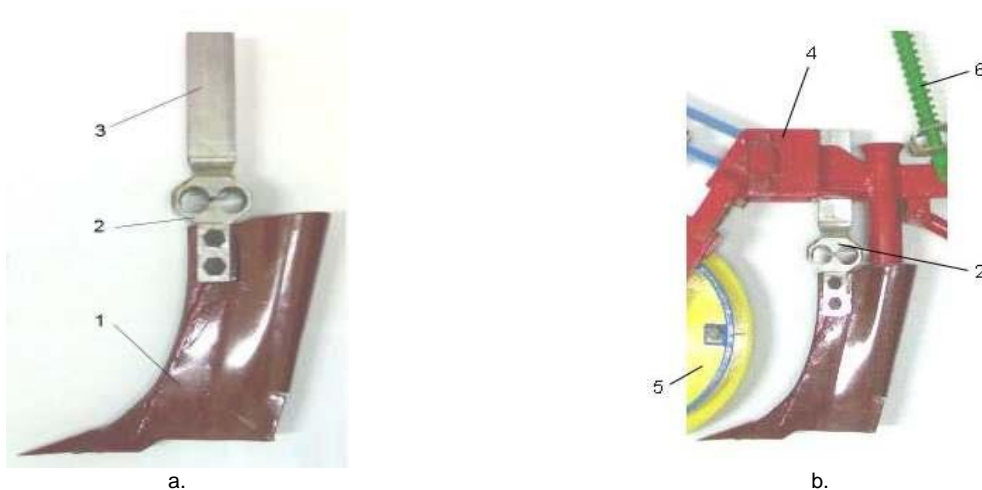
Fig. 8 - Tensometric ring device for determining the forces in fixing arm of soil opener (share) [1, 2]:
