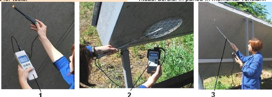
Fig. 2 - Measuring the temperature and the air speed
