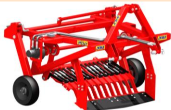
Fig. 1 - Equipment for harvesting Miscanthus rhizomes, ERM
