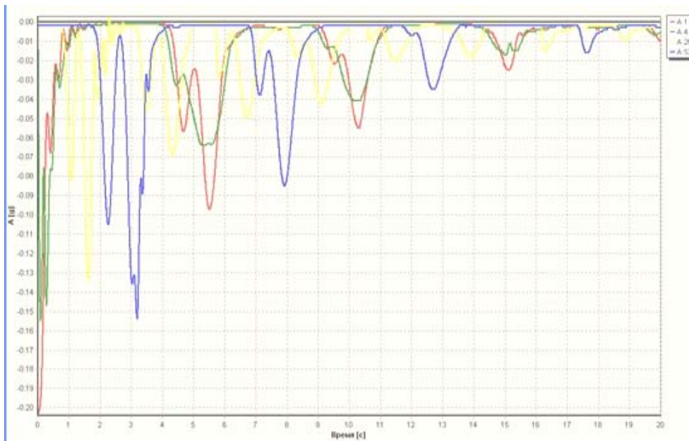
Fig. 7. Oscillograms of longitudinal accelerations of the first locomotive, 4 th , 26 th and 52 nd vehicles at regenerative braking in pre-compacted train
