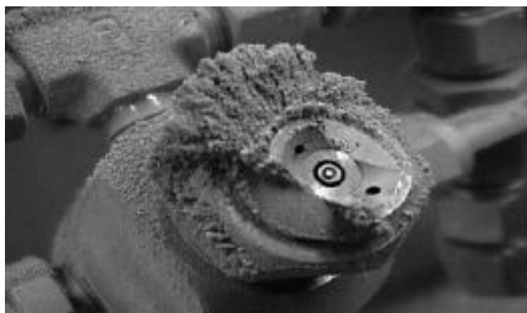
Fig.23: Adhesion of coating material to gun Fi
