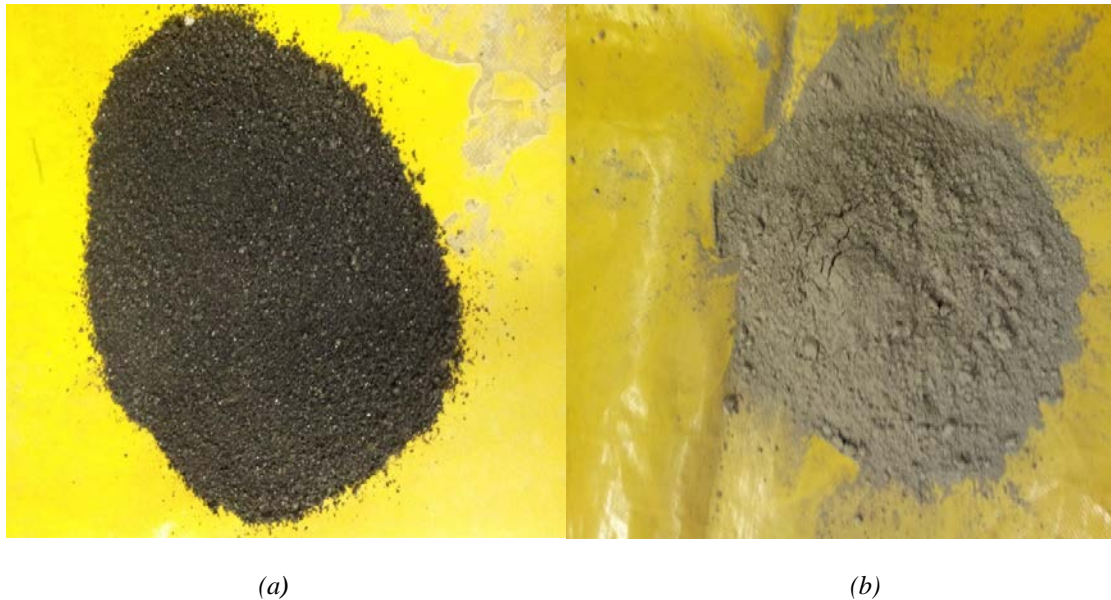
Fig. 1 – (a) Granulated copper slag (b) Pulverized copper slag
