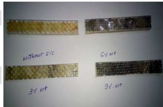
Fig. 2. Flexural test specimen
