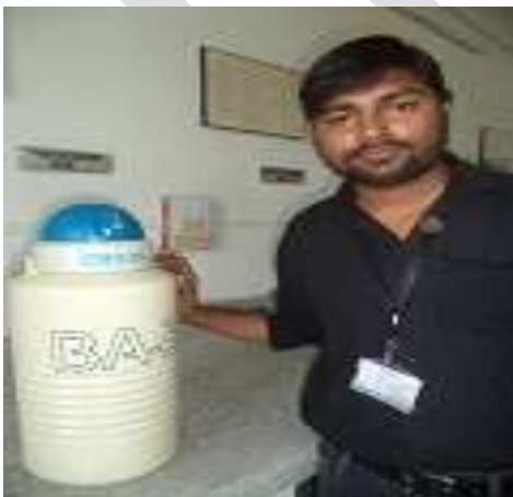
Fig.1 Specimen filled in Cryocan for cryogenic treatment Fig.2 Cryogenically treated specimens of EN24 Steel
