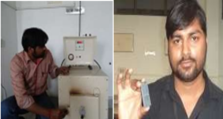
Fig.3 Heat treatment of EN24 Steel in Electric furnace Fig.4 Specimen after Cryogenic Treatment
