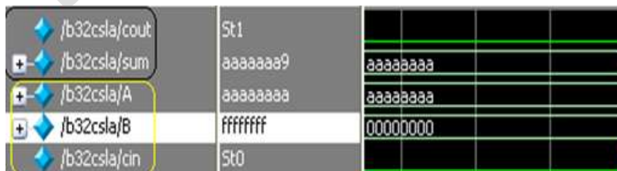
Figure 10: Simulation result of 8-bit modified SQRT CSLA
