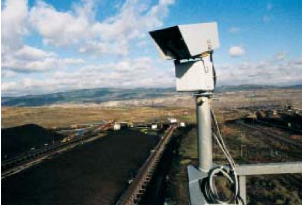
Fig. 1. Infrared camera from FLIR mounted above the coal deposit of the Nástup Mines Cooperation in Tsimice
