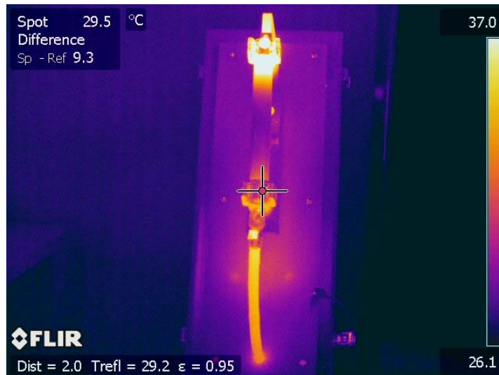
Figure 3. Thermogram of a high voltage switch heated at the superior side [3]
