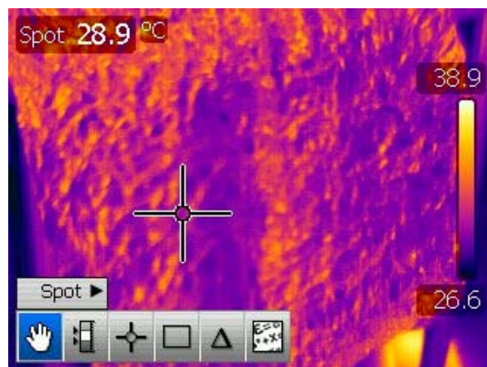
Figure 2. . Thermogram taken with Flir Systems ThermoCam B400 of an aluminum foil which reflects thermal radiation [3]
