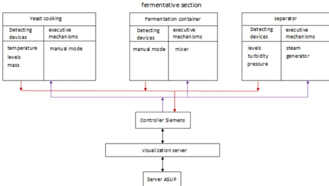
Figure 2 - Block diagram of fermentative section.
