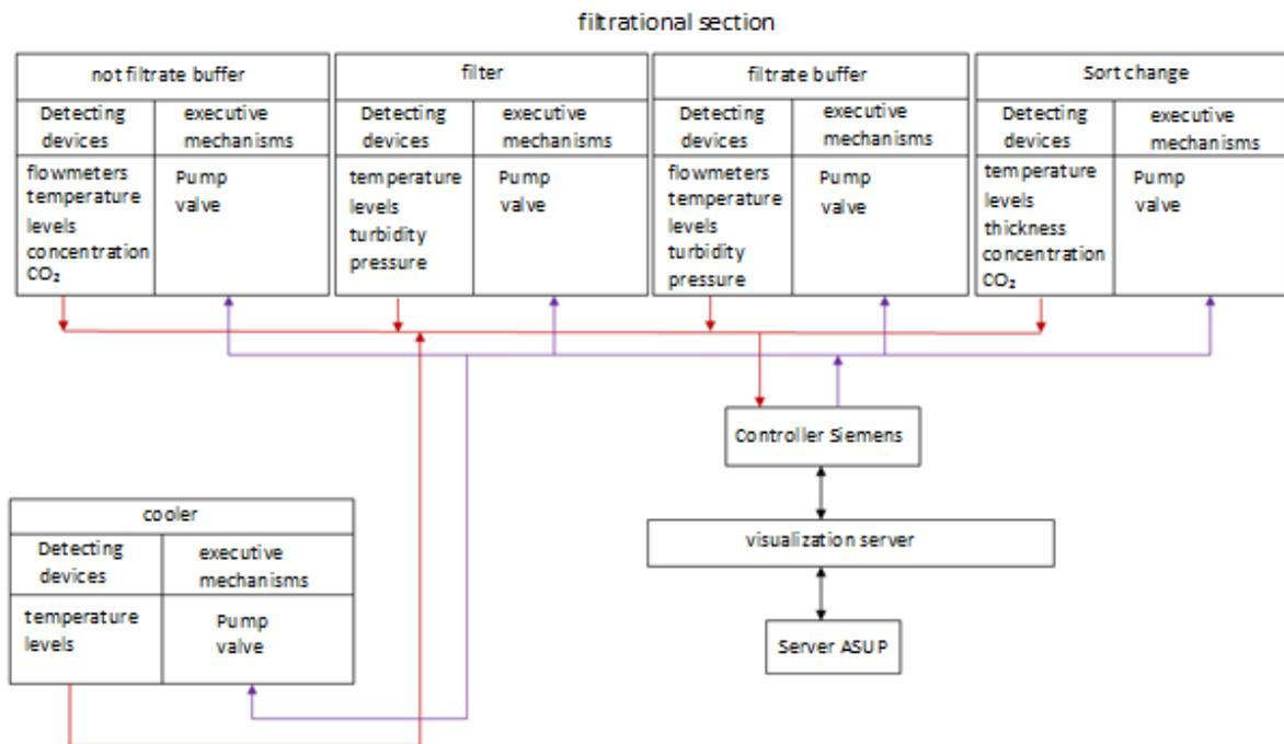
Figure 3 - Block diagram of filtrational section.
