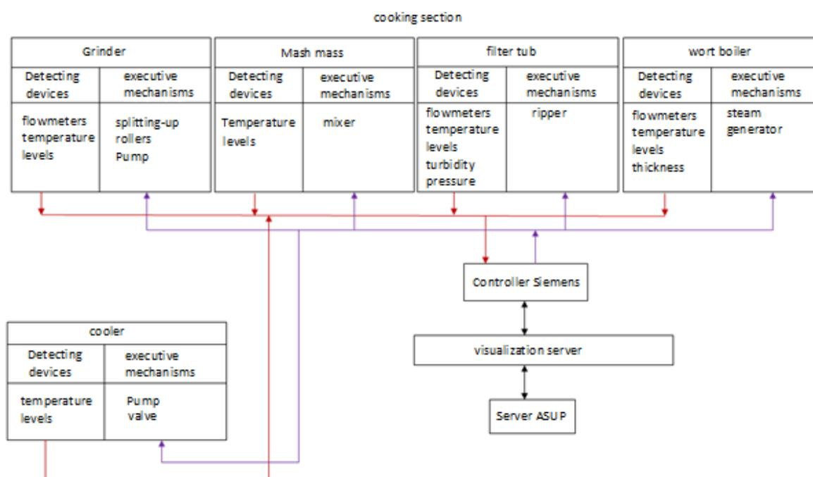
Figure 1 - Block diagram of cooking section.
