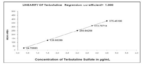
Fig. 3: Graph of Peak Area Vs Conc. of Terbutaline Sulfate.
