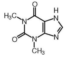
Chemical formula: C<sub>7</sub>H<sub>8</sub>N<sub>4</sub>O<sub>2</sub> Molecular weight: 180.2 Physical appearance: A white crystalline powder. Melting point: 270°C to 274°C Solubility: Slightly soluble in water, sparingly soluble in ethanol (96%). It dissolves in solutions of alkali hydroxides, in ammonia and in mineral acids. Dissociation Constant (pKa): 8.77 @ 25°C.
