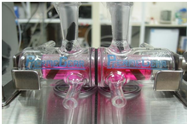
Figure 20: Horizontal /Side-by-side diffusion cell
