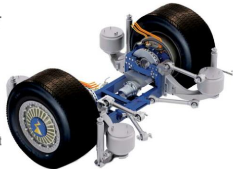
Figure 6 In wheel mounted electric motors [16]
