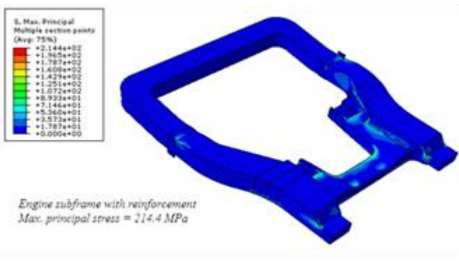
Figure 11. Maximum principal stress distribution on engine sub-frame with reinforcements [17]
