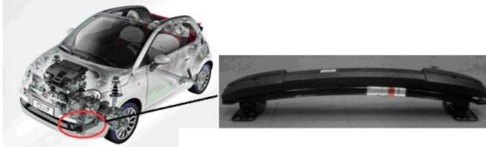
Figure 6 – The present solution for the front bumper system with the bumper beam and the crash boxes made by steel, through the assembly of different parts
