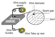
Fig.1. Details of WEDM cutting gap.
