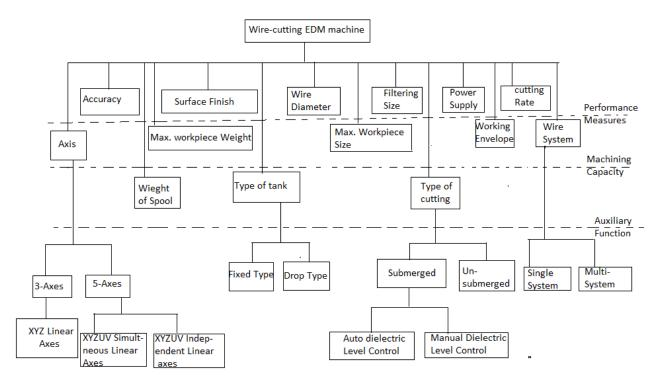
Fig. 4. Classification of WEDM machine.
