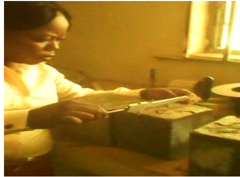
Plate 2: Measuring Cubes Dimension
