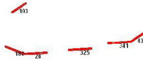
Figure 9: Position of Critical Beam and Column Elements of the Staging in Hydrostatic Case
