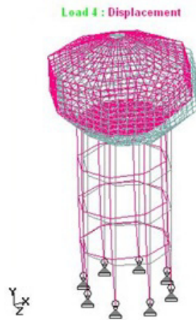
Figure 5: Tank with Its Full Capacity Considering Hydrostatic Forces Along with Sloshing Forces in the Tank
