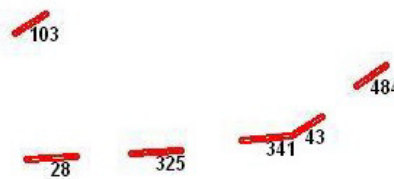
Figure 13: Position of Critical Beam and Column Elements of the Staging in Sloshing Case
