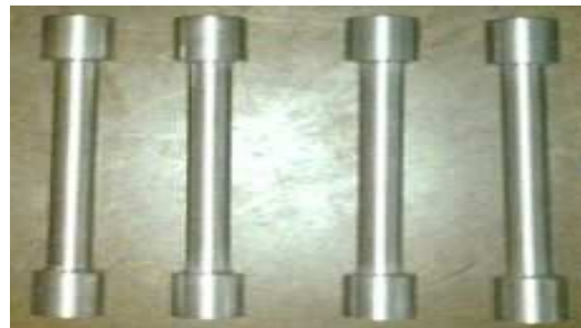
Figure 1: Tensile Test Specimen as per ASTM Standard
