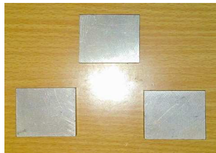
Figure 3: Hardness Testing Specimen as per ASTM Standard
