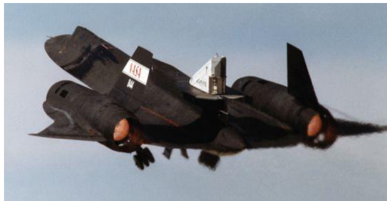
Figure 1.3: Linear Aerospike SR-71 (BLACK BIRD) Experiment (LASRE)
