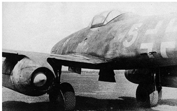
Figure 1.1: First Flight with Plug Nozzle, Messerschmitt Me 262 Germany
