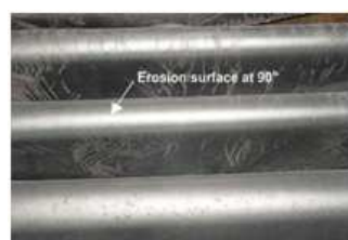
Figure 1: Illustrate Economizer Boiler Tube in a Thermoelectric Power Plant, the Shiny Appearance of Upper Surface Suggested Greater Erosion at 90° Impingement Angle [3]
